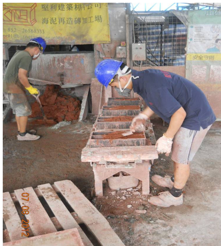
Fig. x Cast MMMM Mixture into Moulds
