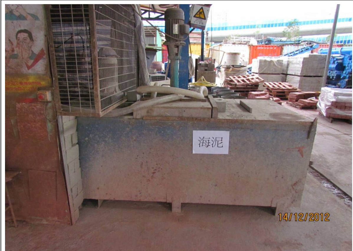
Fig. vi Mix Soaked Marine Mud, Water and Superplasticizer in Pan Mixer No. 2
