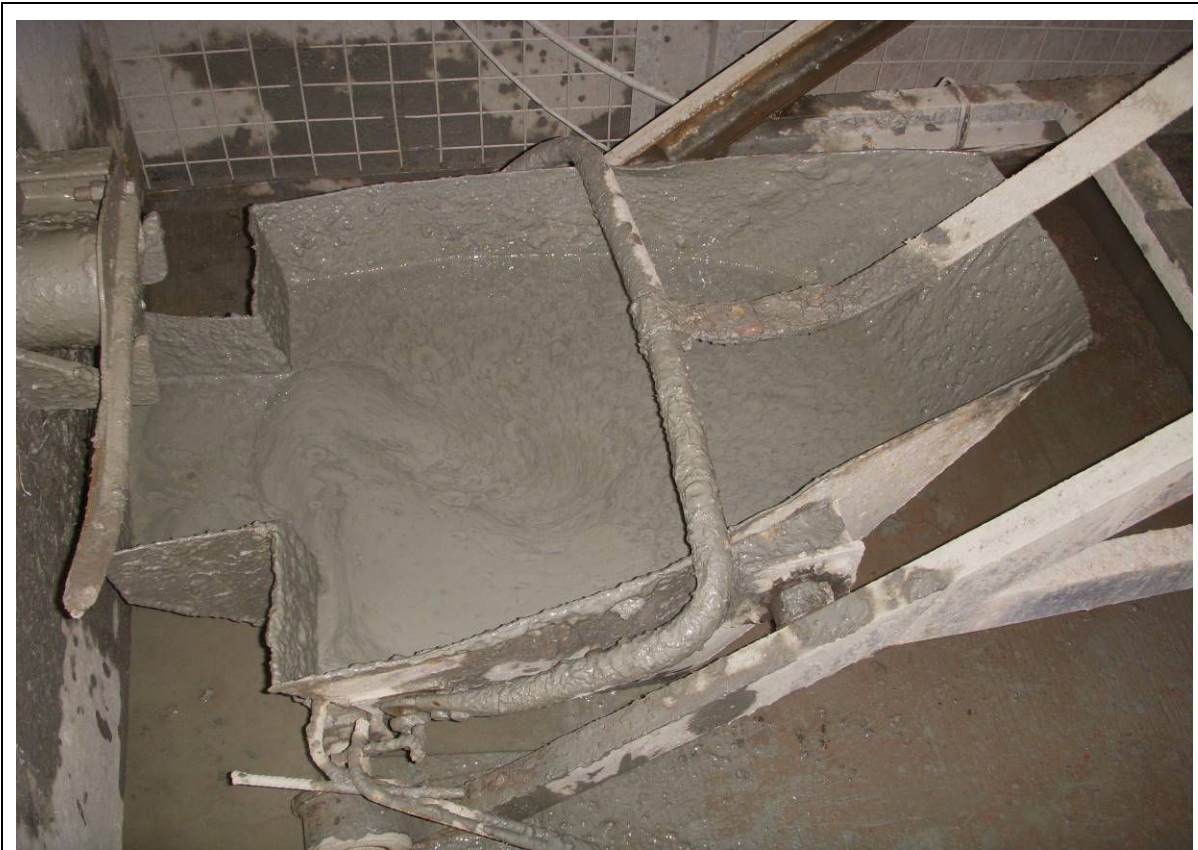
Fig. vii Trowel-able Marine Mud Mix (to be transported from Pan Mixer 2 to Pan Mixer 1)
